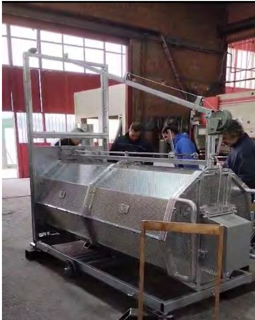
Specially designed culvert trap (specifications from MNP)
