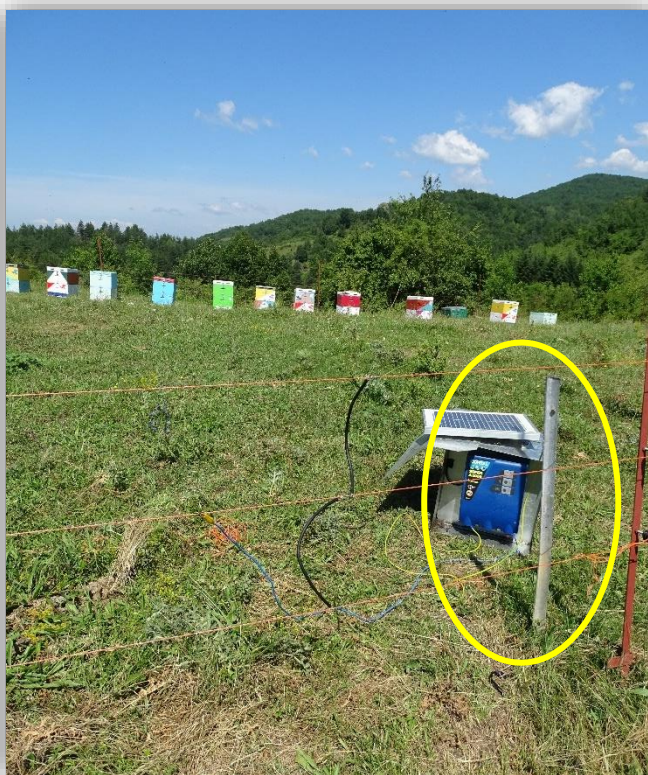
Figures 34-35. In the left figure, the e-fence is incorrectly installed, with the wire positioned on the inside of the corner wooden stake. In the right figure, one can see the grounding is improperly installed, reducing the fence's effectiveness.
