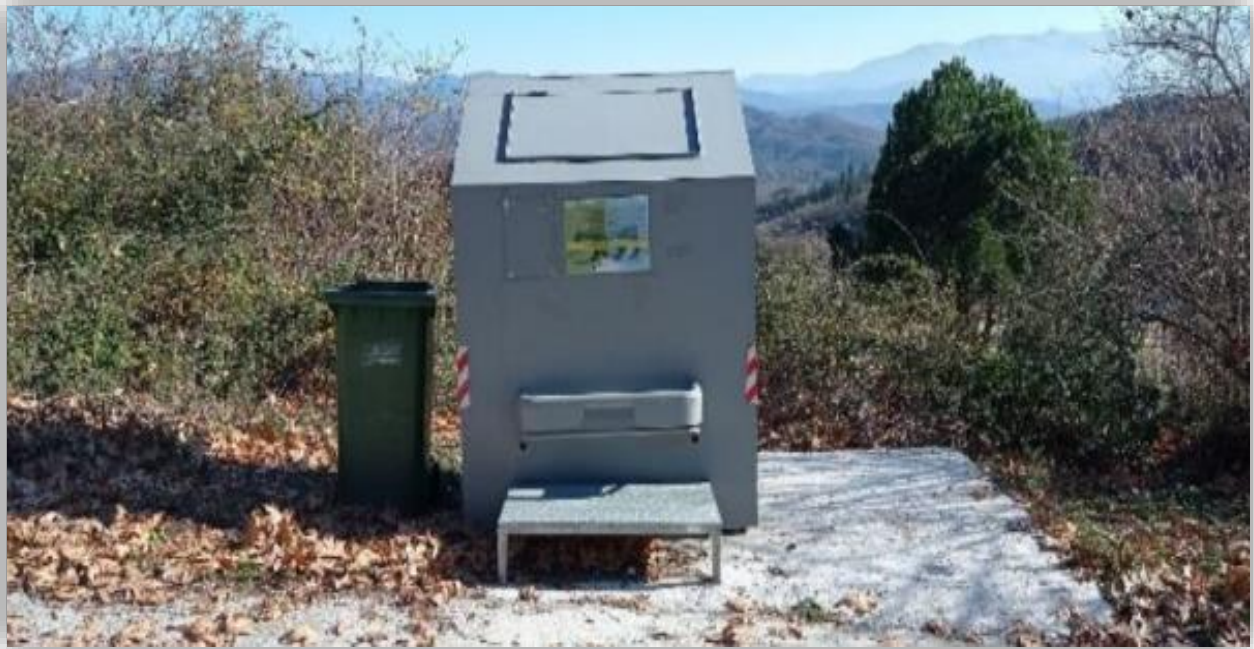
Figure 13. Installation of a bear proof metal shell at Manassis village
