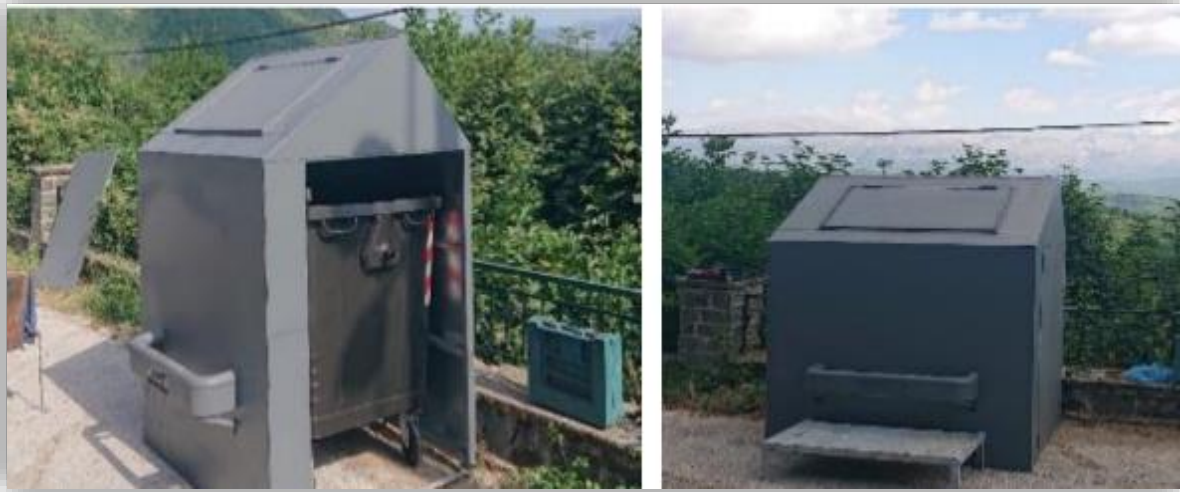
Figures 5-6. Bear proof metal shell protecting a garbage bin installed at Dikorfo village
