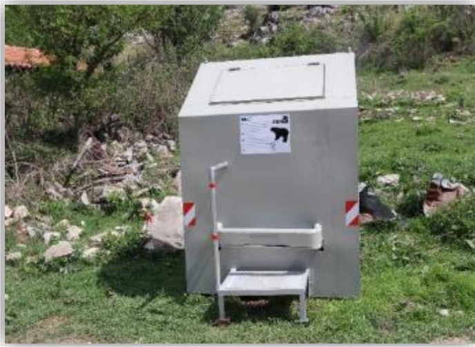
Figure 23. Installation of a bear proof metal shell at Psarades village
