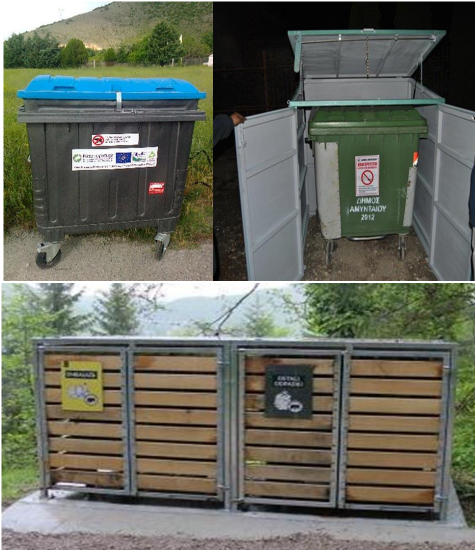
Figure 2-Different types of antibear garbage bins or covers produced under LIFE programs (LIFE09 NAT/GR/000333, LIFE15 NAT/GR/001108, LIFE13 NAT/SI/000550 the latter is used only for biodegradable waste)
