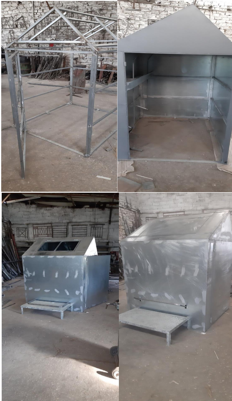
Figure 3-Different stages on the garbage bin cover prototype development
